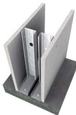
As an example, a double stud partition creating an air cavity eliminates direct mechanical connection between the surfaces. The sound transmission is reduced by breaking the sound path. In addition, the air cavity provides vibration isolation between the two sides. Sound in one room striking the one side of the wall causes it to vibrate but because of the mechanical separation and the cushioning effect of the cavity, the vibration of the other side is greatly reduced.
